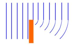
Sea waves incident on a breakwater are found to spread into the region behind the wall where we would expect the sea to be flat calm. This is an example of diffraction at an edge.
